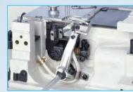
**M**icro-adjuster effortlessly makes fine adjustments for the looper front-to-back position.
