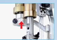
**S**preader holder has alignment mark. Reinstalling the spreader is easy.
