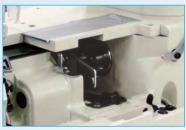
**S**wing in and out looper thread take-up for easier threading.
